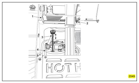
Figure 4-25 Hydraulic Fluid Level Dip Stick
